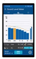
The XL3 determines the frequency spectrum with a Class 1 filter bank in octave or 1/3 octave resolution between 6.3 Hz and 20 kHz. All values are calculated in parallel. In addition, two spectra can be selected and displayed simultaneously. Both the level and the frequency axes can be freely zoomed and scrolled.
