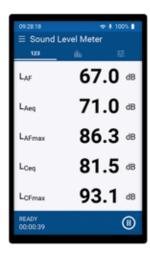
The Class 1 Sound Level Meter records numerous levels in parallel over the entire measurement period. At the same time the XL3 logs the frequency spectrum and, if desired, records the audio as a way file.
