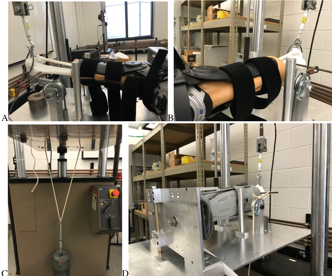
Fig. 1. A) Anterior view of test configuration for eversion of the left ankle with a long TayCo brace. B) Posterior view of the same setup. C) Weights on a cord were used to apply an axial load to the tibia during testing through a pulley system. D) The walking boot was bolted to the foot plate to maintain a rigid connection.
