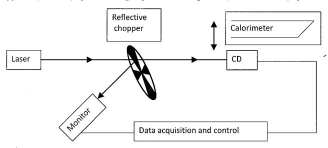
Figure 1. Measurement system diagram.
