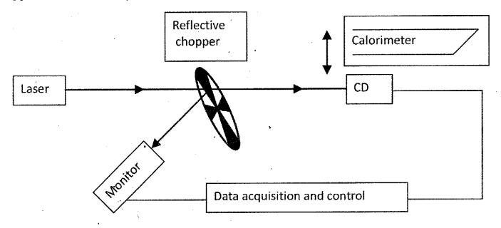
Figure 1. Measurement system diagram.
