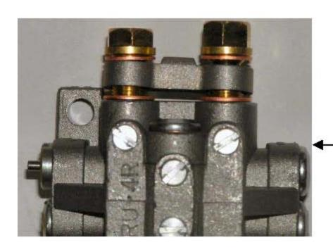
The connector installed (loosely) on the block. Please note the location of the copper washers.
