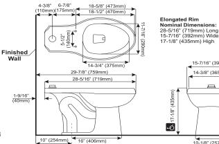
Note: This toilet is designed to rough-in and 12" (305mm) from the wall to the C/L of the outlet.
