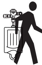
HYBRID.FLUSH ® Flushes When User Leaves
