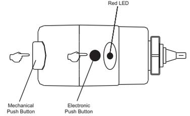
**Red LED** - Constant blinking red LED indicates batteries are low and need replacing.
