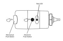
Red LED - Constant blinking red LED indicates batteries are low and need replacing
