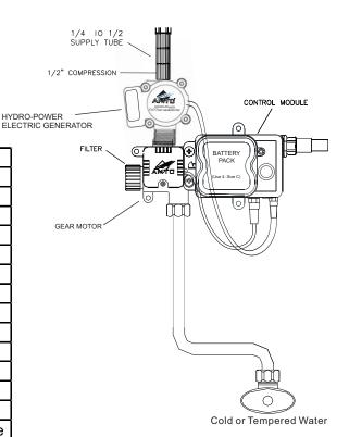
Shown using plug-in hydro-generator.
