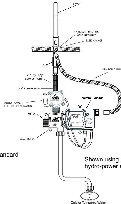
Shown using plug-in hydro-power electric generator.
