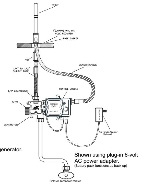
Shown using plug-in 6-volt AC power adapter. (Battery pack functions as back up)
