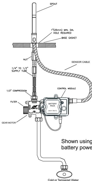
Shown using standard battery power.
