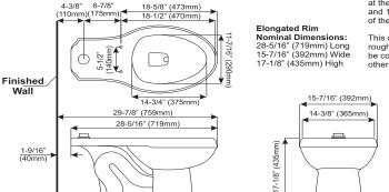
**Note:** This toilet is designed to rough-in at the standard dimension of 10" (254mm) and 12" (305mm) from the wall to the C/L of the outlet.
