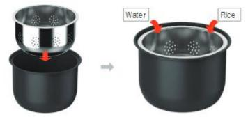
Step 3: Put the water collector flat in the rice container and close the lid cover.
