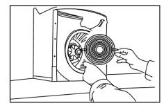
Loosen the screws on the air inlet ring and then take it out.
