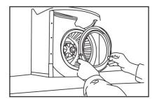
• Turn the locking nut in clockwise direction to take out the impeller for cleaning.
