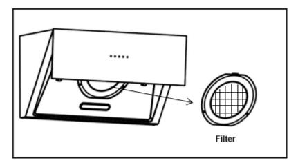
• Loosen two screws around the air inlet ring and install the charcoal filter.
