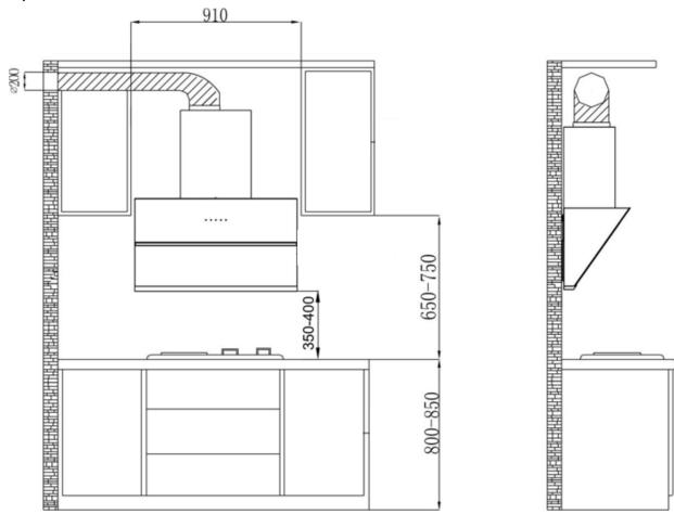
Before installing, determine the height between the bottom of the cooker hood to the top of the hob. Mark on the wall to suit the bracket locations.
