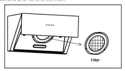
Loosen the screws on the charcoal filter and then take it out.
