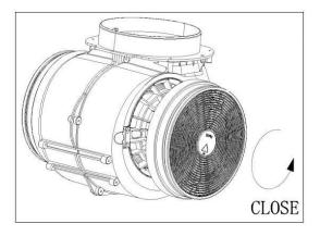
• On the right side, Install the charcoal filter and lock the position by turning clockwise direction to tighten.
