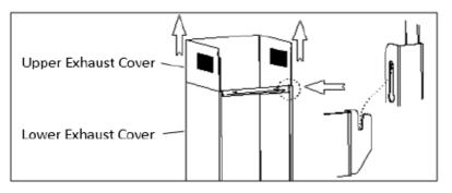
• Drill 2 holes with diameter of Ø8mm. Insert the screw anchors into the holes. Fix the mounting bracket and tighten the screws.
