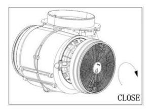
• To remove the charcoal filter, reverse the direction on above direction to loosen.
