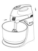
Align the hole at the bottom of the hand mixer with the clips on top of the upper base, and then press the base switch to assemble the hand mixer to the upper base until it "clicks".
