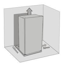
6. Allow the side of the appliance keep at least 50mm distance when installing and allow the door be open  $135^{\circ}$
