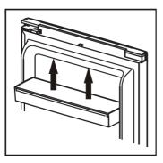
4. Pull out the fresh zone to stopper position. Lift up the front and then pull out.
