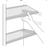
3. Remove each balcony / rack by lifting up and pull out slowly.
