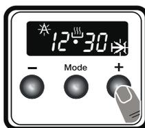
3. Use the "+" and "-" buttons to set the desired finishing time.
