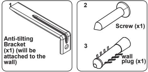
The document bag contains an anti-tilting kit. Loosely attach the anti-tilting bracket (1) to the wall using the screw (2) and wall plug (3), following the measurements shown in the figure and table below. Adjust the height of the anti-tilting bracket so that it lines up with the slot on the cooker and tighten the screw. Push the appliance towards the wall making sure that the anti-tilting bracket is inserted into the slot on the rear of the appliance.
