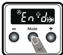
5. Press **"MODE"** until you see **"end"** and
