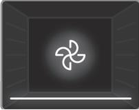
**Lower Heating and Fan Function:** The oven's thermostat and warning lights will switch on, and the lower heating element and fan will start
