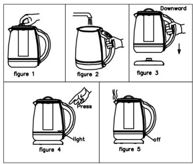
Before using the appliance for the first time, water should be boiled in 2 times without any additives.
