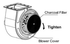
To remove the charcoal filter, turn anti-clockwise direction to loosen.
