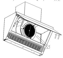
Install the charcoal filter and lock the position by turning clockwise direction to tighten.
