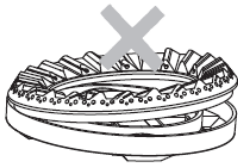
Burner ring is not positioned properly
