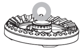
Burner ring is placed correctly
