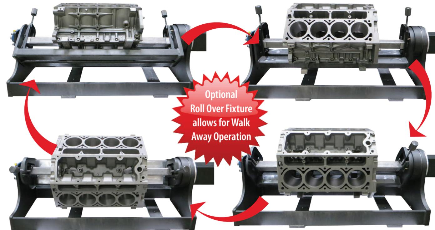
Optional Roll Over Fixture allows for Walk Away Operation
