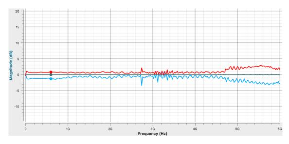
Measurement of calibration standards (OSL) at environmental temperatures of -20°C (blue), RT(green) and +85°C (red) without re-calibration:
