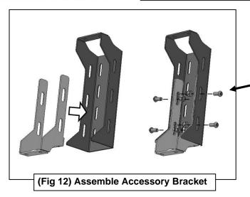
(4) 8mm x 20mm ButtonHead Bolts(4) 8mm Nylon Lock Nuts
