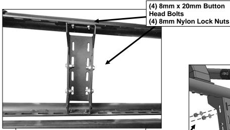
(Fig 14) Accessory Bracket installation pictured from back of Rack
