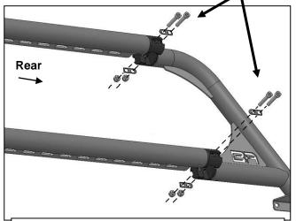
(Fig 6) Attach Side Tube to Rack End assembly (NOTE: Fully install lower tube first).
