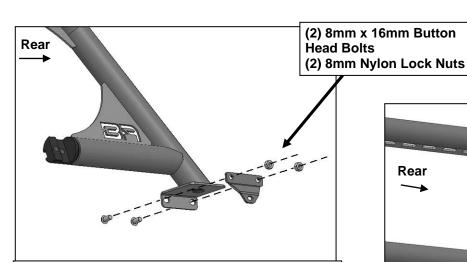
(Fig 5) Attach (1) rear Mounting Bracket to bottom of the driver/left rear Rack End Assembly
