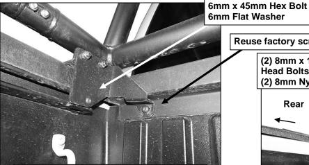
(Fig 10) Attach driver/left front Mounting Bracket to side and front of bed (arrows)
