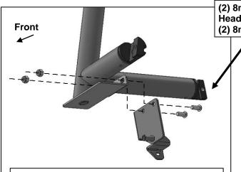
(Fig 1) Attach driver/left front Mounting Bracket to bottom of Rack Corner Assembly
