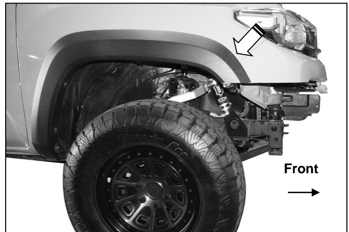
(Fig 17) Reuse the factory fender bolts to attach the front Fender Flares (passenger/right side pictured)
