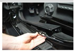
Remove the floor plugs under the seats. Drop the motor connector (D & N) through the open holes.
