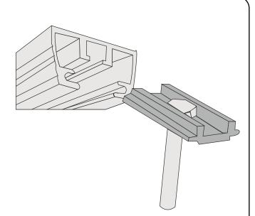
At each of the four corners where the rack bars and mounting tracks cross, using a steel mounting plate and nylock nuts to secure the bolts on either side of the bar. Tighten all eight bolts securely with the included nuts and wrench. Check all the mounting bolts and brackets periodically during use.
