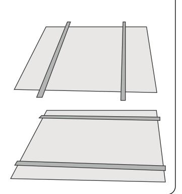
Slide the 10mm nylock nuts into the inner slot in the center of the mounting tracks until they are aligned with the holes in the mounting tracks and the base.
