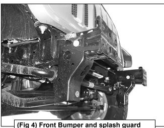
(Fig 4) Front Bumper and splash guard removed from 2018-on JL model pictured
