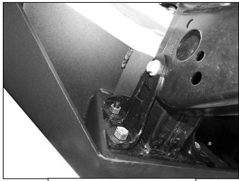
(Fig 12) Driver/left side of Bumper installed on JL model
