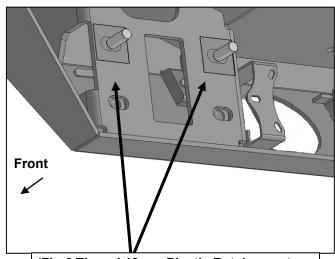
(Fig 6 Thread 12mm Plastic Retainer onto Bolt to hold Bolt/Nut Plate in position
