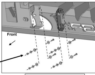
(Fig 8) Attach 4-bolt Fog Light to mounting plate and Adapter
