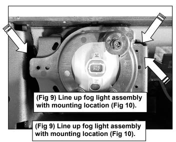
Attach offset style fog light from JL Sport model w-1pc plastic bumper, directly to mounting plates. Driver/left side pictured
