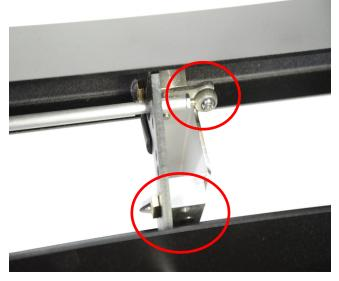
Deploy the steps, pressure wash the bodies clean including internals, then apply a multipurpose lubricant to each of the areas as shown.
