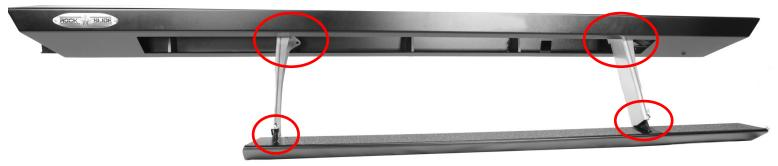
You will need to lubricate the pivot points that are circled in red shown above.
