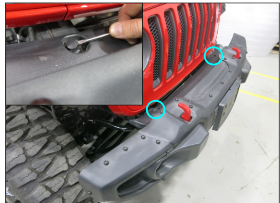
4. Remove fascia plate trim clips. Remove plastic push clips, using a small feather edge screwdriver.
