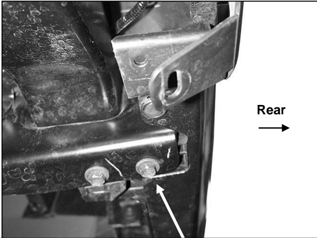
(Fig 6) Models with receiver hitch, remove the hex bolts attaching bumper to bottom of hitch
