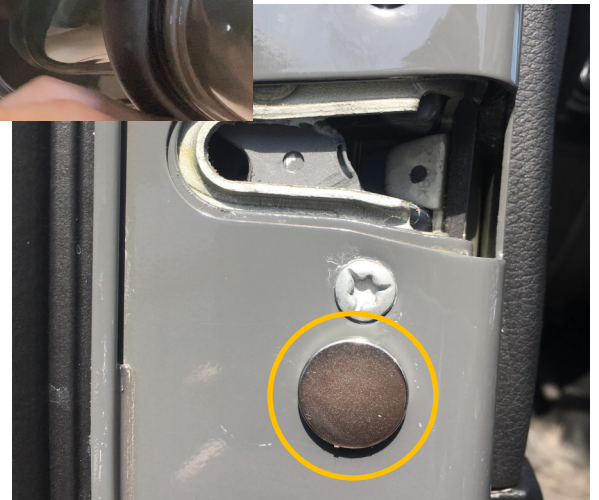
Front Door Magnet Placement
