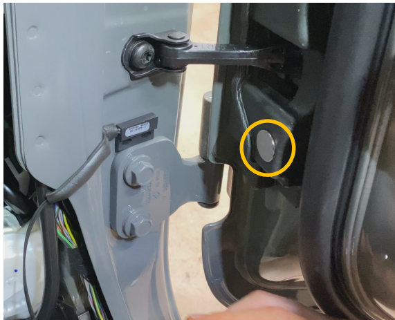
Rear Door Magnet Placement
