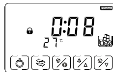
Ice full standby
