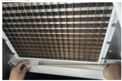
8. While soaking the parts, use a nylon brush or soft cloth dipped in cleaning fluid to wipe the surface of the parts that are in contact with water and ice, such as evaporator ice trays, ice shields, ice storage buckets, etc. The damp cloth wrapped disposable chopsticks to clean up). Then rinse with clean water (rinse 5 times).
