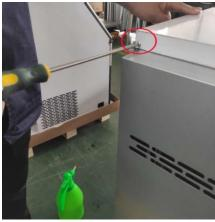
Lift the top cover slightly upwards first, and then gently pull back to pull out the top cover
