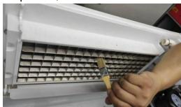
Use nylon brush dipped in descaling agent or vinegar to scrub the plastic parts around
