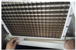
While soaking the parts, use a spray can to evenly and completely spray the disinfectant on the surface of the parts that are in contact with the ice, such as the evaporator ice tray, ice shield, ice storage bucket, etc. (the dead corners can be wetted with disinfectant Disposable chopsticks wrapped in a rag to
