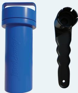
If you notice air leaking from the valve, this is easy to fix using the supplied spanner in your repair kit. Remove the valve dust cover and insert the crown shaped end of the spanner into the valve. Turn the spanner clockwise until tight to reseal.
