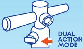
2. For quicker inflation, use the dual action mode. You can toggle between dual and single action with the selector switch (or bung) on the side of your pump.
