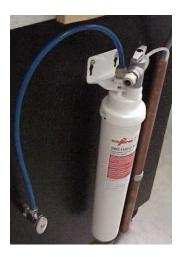
5. Connect metal braided water hose from espresso machine to filter using 1-2 feet of 3/8 inch blue plastic tubing.
