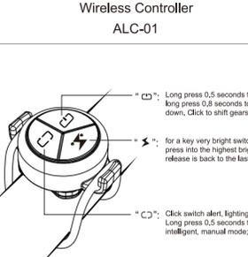
Fixed to the handlebars by a o-ring strap, contain a replaceable CR1632 button battery.
