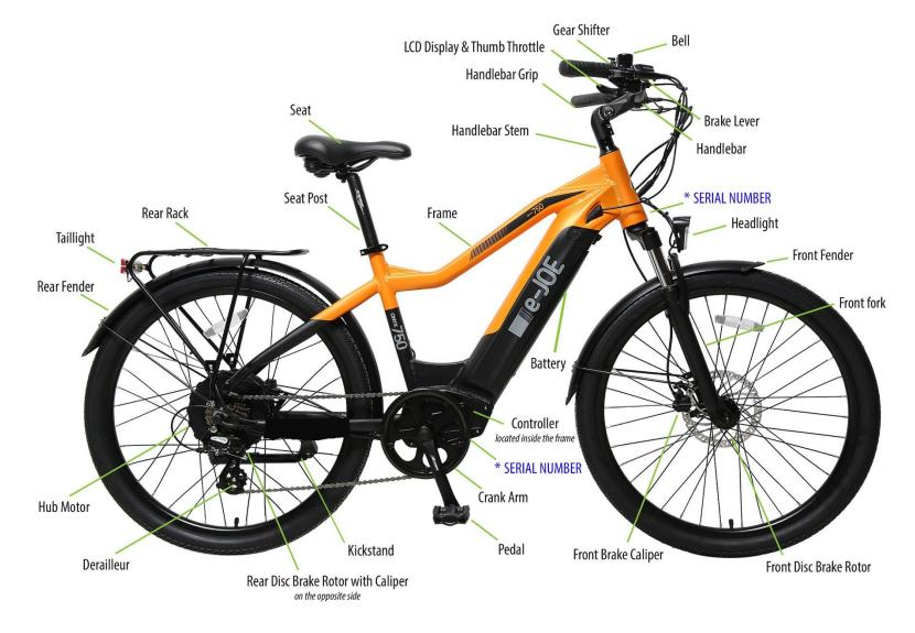
\*The serial number of the electric bike is printed either on the headtube of the frame above the front suspension fork or on the bottom of the downtube between crankarms. The regular format is AB01234567.
