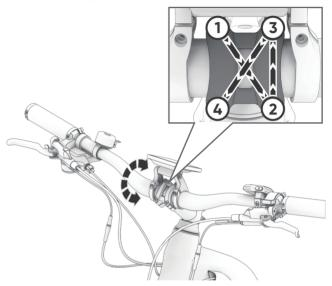
Loosen the front bolt on the stem and adjust the handlebar to the right angle
