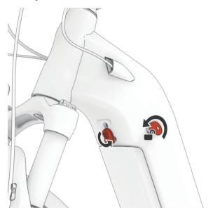
Insert the key and turn left to open the first lock. While holding the top of the battery with your hand, turn the safety lock in the direction of the arrow shown with the other hand.
