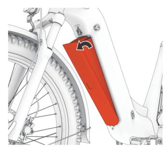
As shown in the picture, carefully remove the battery.
