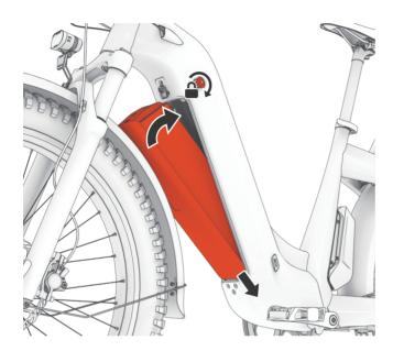
When installing the battery, first insert the low end of the battery into the internal slot in the bottom of the downtube smoothly. Then push the upper end of the battery into the downtube and turn the key to the right to lock it.
