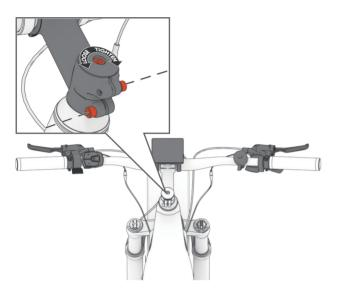
Loosen the screws on the stem and stem cap, push the front wheel against the wall, and adjust the direction of the stem so that it is in line with the front wheel. Make sure the handlebar is perpendicular to the front wheel and press down on the handlebars and tighten the stem cap screw. Finally, make sure that the handlebar is perpendicular to the front wheel and tighten the screws on both sides of the stem.
