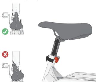
Open the seatpost quick release lever and adjust the seat to the proper height, then close the lever. If the seatpost continues to slide down, please screw the adjusting bolt on the seat clamp.
