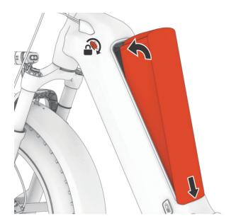
When installing the battery, first insert the low end of the battery into the internal slot of the downtube to ensure that the terminals at the bottom of the battery are smoothly inserted into the slot inside the downtube. Then push the upper end of the battery into the downtube and turn the key to the right to lock it.
