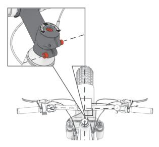
Loosen the screws on the stem and stem cap, push the front wheel against the wall, and adjust the direction of the stem so that it is in line with the front wheel. Make sure the handlebar is perpendicular to the front wheel and press down on the handlebars and tighten the stem cap screw. Finally, make sure that the handlebar is perpendicular to the front wheel and tighten the screws on both sides of the stem.
