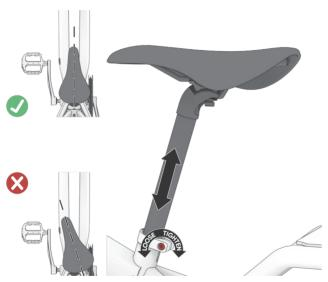
Loosen the adjusting bolt of the seat clamp and adjust the seat tube to the appropriate height. Then lock the seat clamp and make sure the stationary ladle faces forward.
