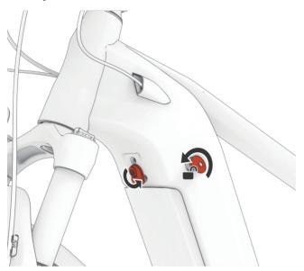
Insert the key and turn left to open the first lock. While holding the top of the battery with your hand, turn the safety lock in the direction of the arrow shown with the other hand.
