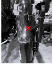
**Step 3** – Insert the supplied Allen bolts through the knuckle and mount the light onto the side of the knuckle. Mark the location to drill the hole for the wire. **X** in the picture shown. You will only use the supplied black Spacers for RAPTOR and BLADE installs for Pro II and Sportsman II do not use spacers.
