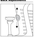
Lumbar height adjusts 5" (51/4" to 101/4" from seat, 61/2" to 111/2" on Plus chairs) by grabbing exposed tabs and sliding the lumbar support up or down. This feature is standard on work chairs and stools, but may be omitted.
