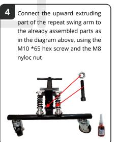
(1) tighten securely with the 8mm hex key and spanner provided.
