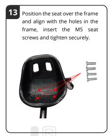
We recommend using the thread locker provided, as the screws and nuts can become loose overtime with the vibration. Regularly check and tighten acres and nuts,
