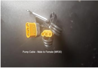
Figure 23 Pump to ECU Cable
