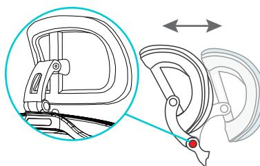
Press the button,it can be adjusted forward and backward.
